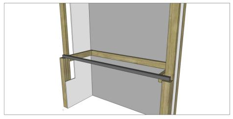
The sink will float by resting on 3 wall cleats: Left, Back, Right. The front of the sink will be supported by a properly gauged tube steel bar. The bar will sit on wall blocking and be screwed into the studs.
