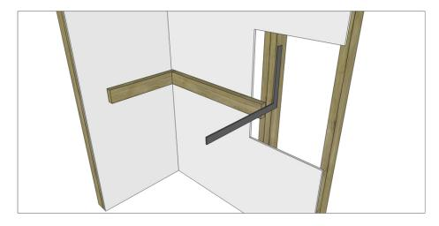
The sink will float by resting on one Floating Sink Bracket (L or T). The side & back wall will rest on wall cleats.
