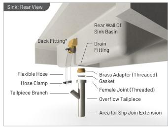
\* The Front Fitting threads into the Back Fitting and seals internally with an 0-Ring. Set Screws (on the Rear Fitting) tighten against the back of the sink to compress a second 0-Ring that rests between the Front Fitting and sink.
